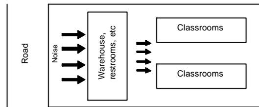
**Figure 1:** The use of "buffer zones" to minimise noise and allow natural ventilation.
