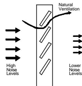
**Figure 2:** Example of an acoustic louvre. Section.
